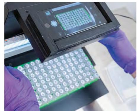
The sample position on the plate is photographed and recorded using the QR code.
